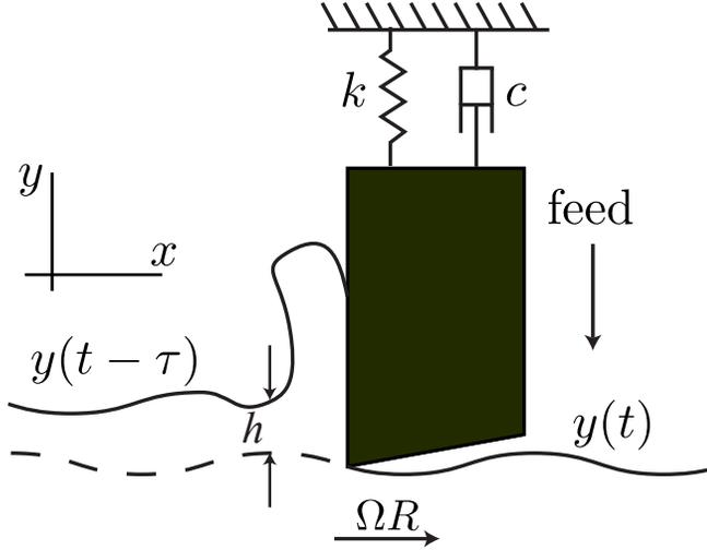
**FIGURE 3.** The turning process under study in this paper. The tool is compliant in  $x$  while the workpiece is assumed rigid.
